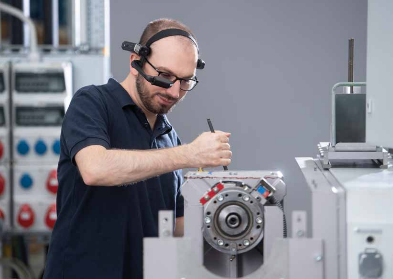
Esref Halil demonstrates the data glasses in the Extrusion Engineering Service Center. With the video communication from expert to user, service activities can be supported visually and guided step by step.
