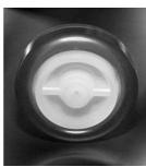
PUR part produced from two components, a harder PUR core and a smoother PUR membrane that are chemically combined by a casting process
