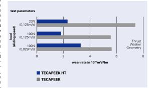
Wear resistance of TECAPEEK HT compared to TECAPEEK at different parameters
