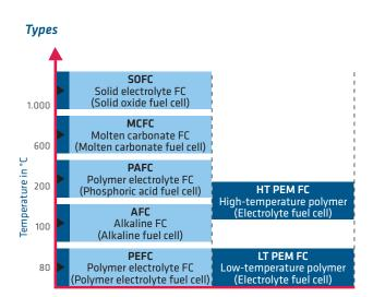
LT = Low-temperature, HT = High-temperature, FC = Fuel cell
