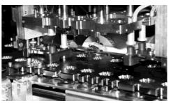
Hold-down plate made of TECAPEEK ELS
