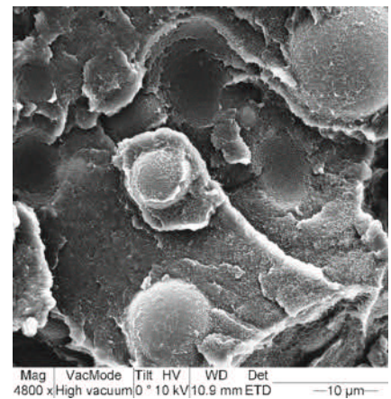
Fig. 6. SEM: in the material Tecacomp LW, the hollow glass microspheres are optimally bonded to the polymer matrix, which results in increased mechanical performance (figure: 3M)
