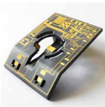
Fig. 5. Three-dimensional micro-component onto which very fine interconnect structures have been applied by laser direct structuring (figure: LPKF)
