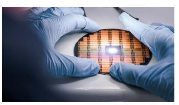
With TECAWAFER, Ensinger offers a 4-inch wafer as an alternative to wafers made from silicon, ceramic or glass. The patented polymer-based Ensinger Microsystems Technology (EMST) enables individual adaptations which can be implemented cost-effectively even in small quantities.
