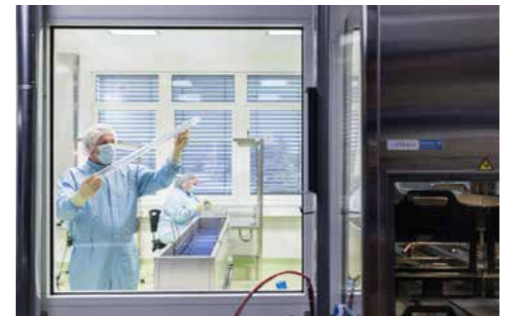
The machined parts pass through a rinsing sluce (right) into the cleanroom where they are assembled and packaged. Large items such as the component for a bioreactor shown here are rinsed in a trough with highly purified water.
