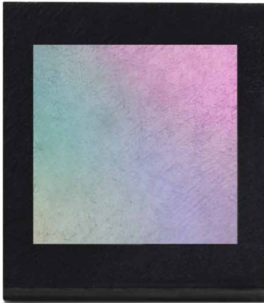
The illustration shows microstructures (Bragg grating) on a sensor. The compound TECACOMP PEEK LDS black 1047045 made by Ensinger is extremely temperature-resistant, has very good weld line strength, good adhesive strength and shows very high chemical resistance to solvents. Furthermore, the material has a very low coefficient of linear thermal expansion. Photo: Ensinger / IMPT
