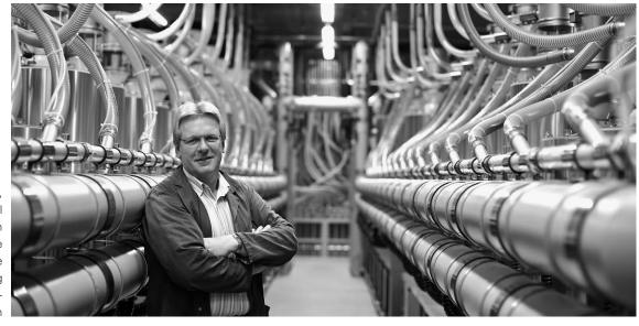
Thomas Musch, Head of Material Processing – from here the granulate is transferred to the injection moulding machines via a distribution system
