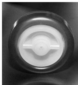
PUR part produced from two components, a harder PUR core and a smoother PUR membrane that are chemically combined by a casting process
