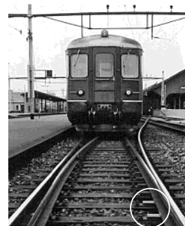
The gliding parts are formed in dovetail shape. Diagonally to the gliding direction there are notches that drain off wear dust and dirt particles.
