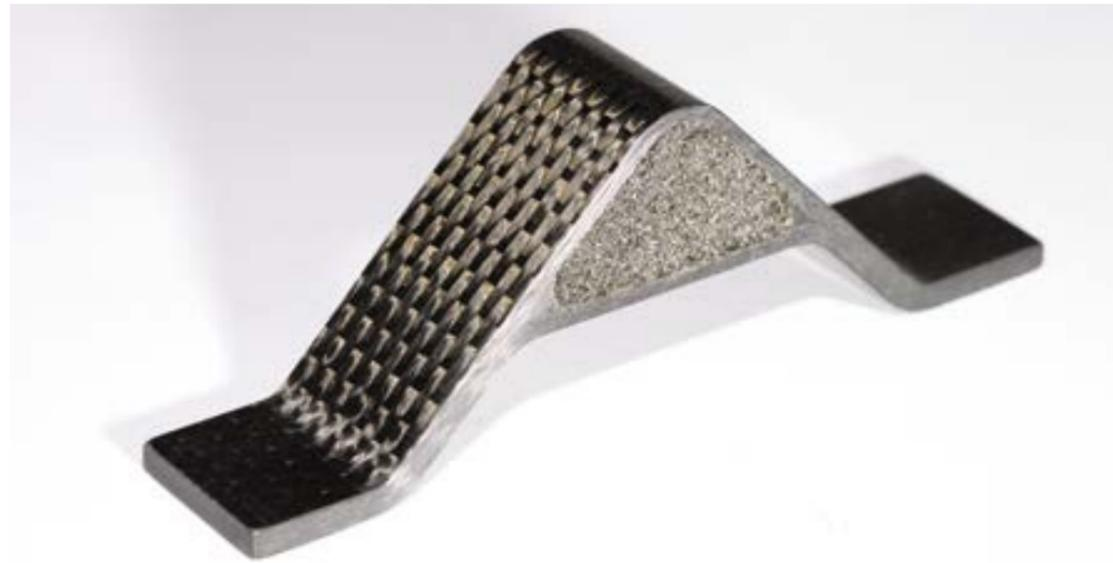
next composites develops technologies for processing thermoplastic fibre composite materials. The sandwich profile shown above was made of CF-PEI and recycled foam glass (cross-section).
