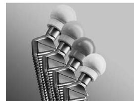
Sizing trials for hip implants. For this application material has to be low-stress and non-warping. It also needs to be resistant to multiple sterilisation and cleaning agents. Different colours allow easy differentiation of sizes. TECAFORM AH MT was selected since this thermoplastic fully meets these requirements and is available in a large range of colours.
