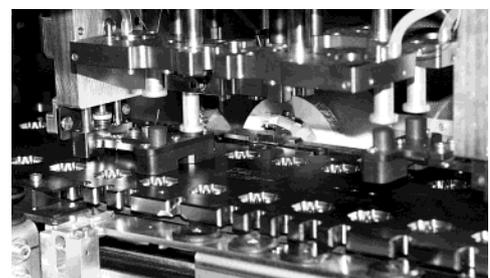
Hold-down plate made of TECAPEEK ELS
