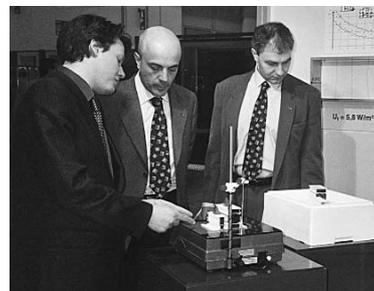
The chocolate experiment: Chocolate, separated by insulbar® profiles from a +35 °C hotplate, melts if the profiles have a low size. A larger size (triple tubula insulbar® with very thin walls) prevents from melting, since that way a better thermal insulation can be achieved.
